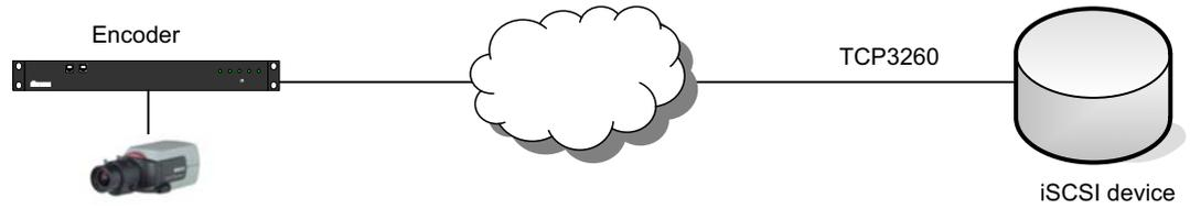
**Figure 6.5** Open ports for Direct-to-iSCSI recording
